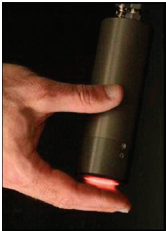
FIGURE 2.5.1 The control of atmospheric pressure plasmas will provide the ability to economically treat complex surfaces, up to and including living tissue. Courtesy of R. Hicks, SurfX Technologies LLC.
