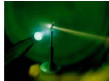
Photograph of the LLNL Petawatt laser striking a solid gold target and producing a cone of accelerated electrons and protons with energy up to 100 MeV. The laser enters from the left.
