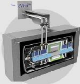
eVinci Heat pipe-cooled microreactor WESTINGHOUSE NUCLEAR
