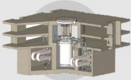
KP-FHR Fluoride salt-cooled high-temperature reactor KAIROS POWER
