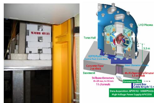
Figure 2. (left) Neutron collimator installed in NSTX (right) Neutron camera in LHD. Reproduced with permission from K. Ogawa et al., Rev. Sci. Instrum. **89** (2018) 113509.
