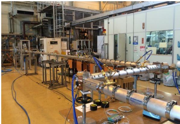
Figure 1. Transmission Line test set-up at QST, where a 1MW, 170 GHz gyrotron, located in the large enclosure at the back wall, is used to test components on the transmission line
