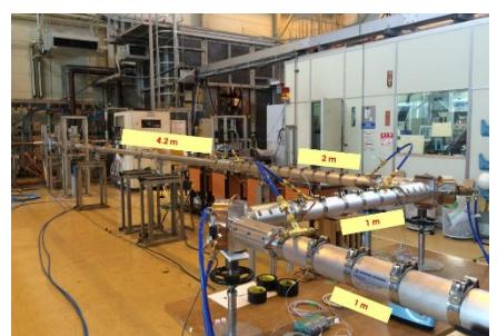
Figure 3. The arrangement of water-cooled waveguides, including the 4.2-m waveguide assembly and the expansion joint, in the transmission line.
