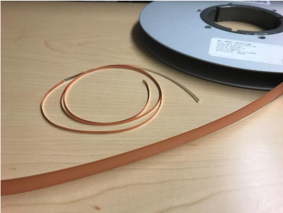
Figure 4.2.1. Two commercial tapes from SuperPower: 12 mm wide, 100 μm thick tape and 2 mm wide, 45 μm thick tape.
