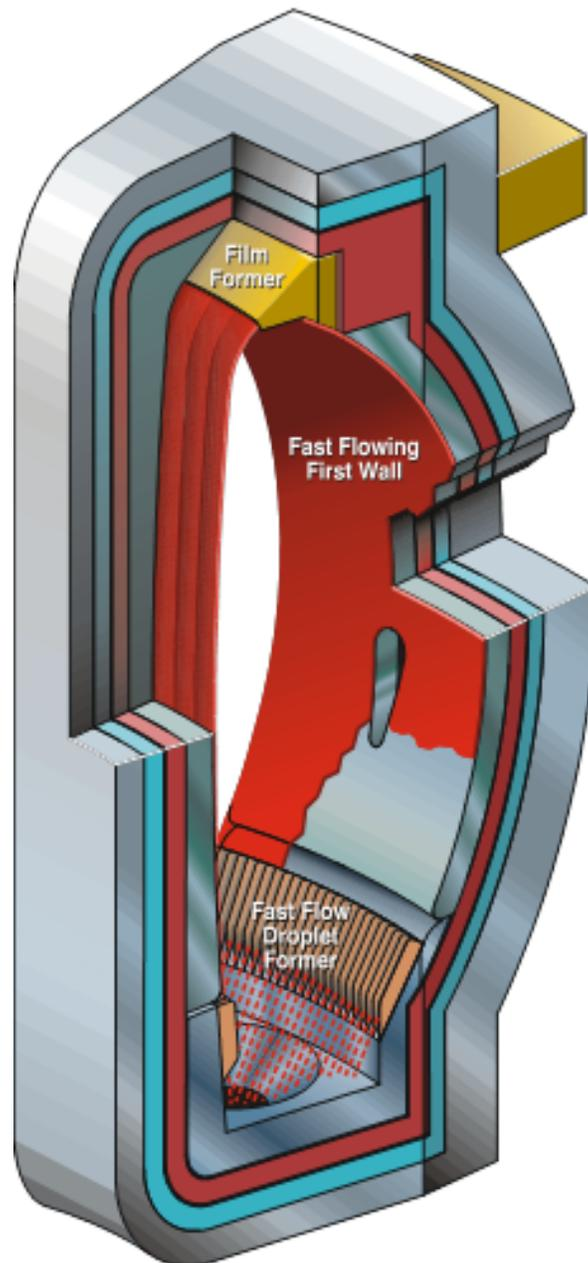
CLIFF Convective Liquid Flow Firstwall
