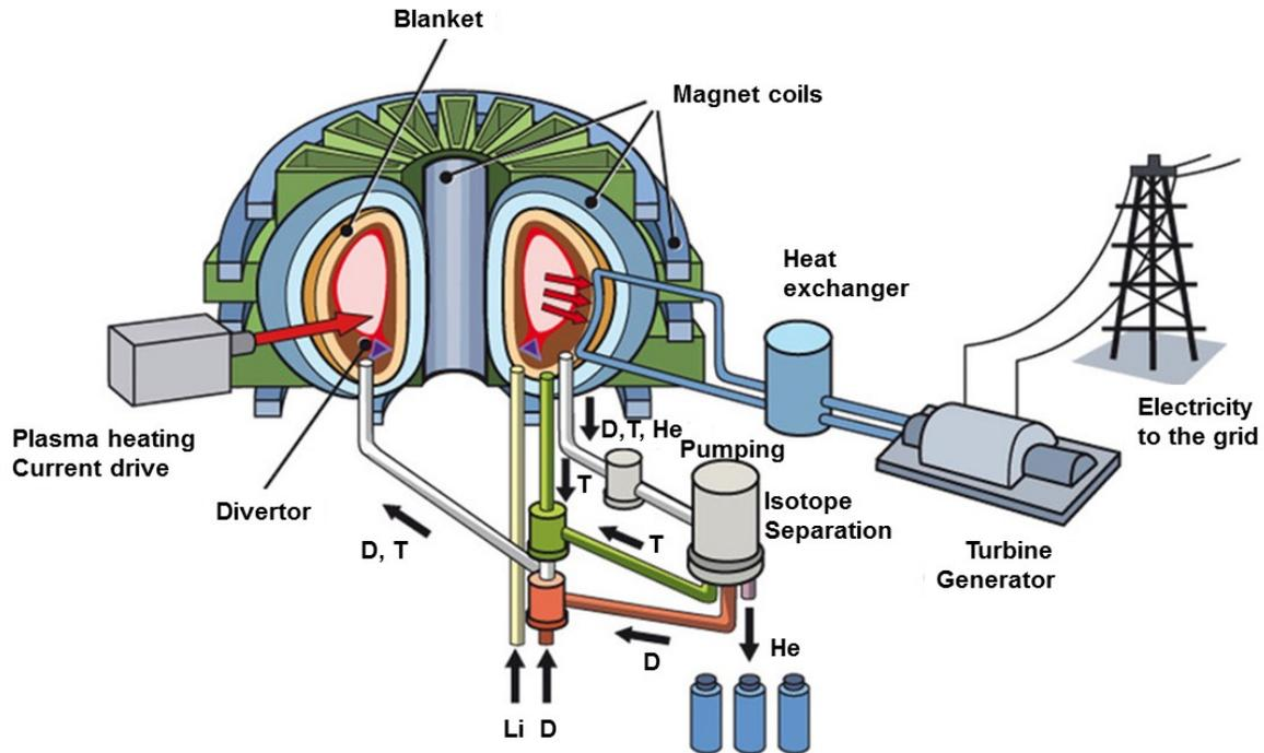
Layout of a future tokamak fusion power plant © IPP,
