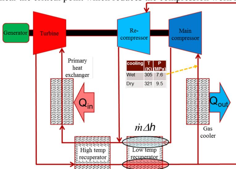
Figure 6.7.1. Supercritical CO<sub>2</sub> Recompression Closed Brayton Cycle diagram: the flow is split at points to optimize the thermal capacities of the heat-exchanging streams.
