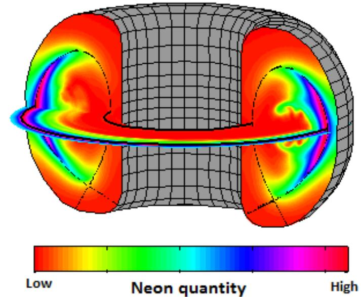
Concentration of edge-injected Ne impurity after dynamic mixing, as predicted by integrated nonlinear simulation, combining 3D MHD and radiation modeling. Image courtesy of V. Izzo (UCSD).
