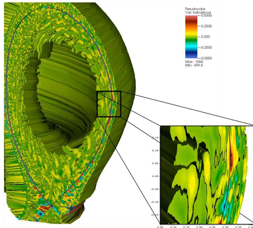
Contours of turbulent electrostatic potential from an XGC1 5D (3r,2v) gyrokinetic simulation that spans the pedestal and SOL in DIII-D magnetic geometry.
