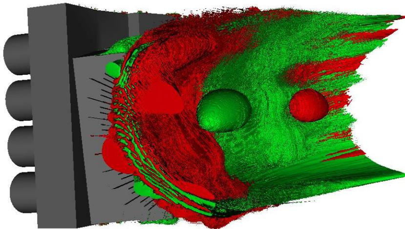
**Contours of the vertical electric field induced by the field-aligned ICRF antenna in the Alcator C-Mod device. Both fast waves (large blobs near reactor core) and slow waves (short-wavelength behavior near plasma-facing antenna surfaces) are present. Image courtesy of T. Jenkins (Tech-X).**
