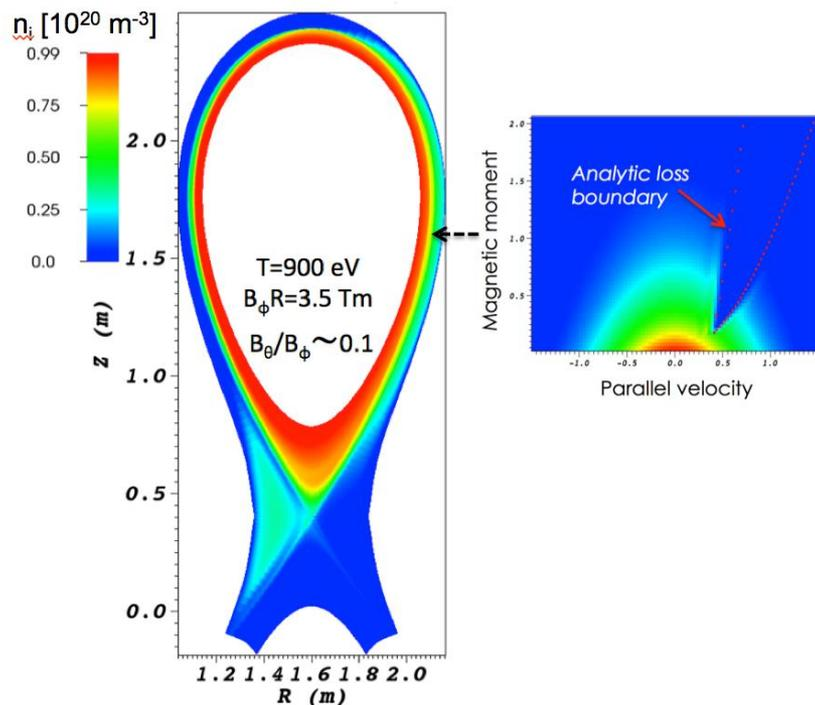
COGENT 4D (2r,2v) kinetic simulation showing ion density and velocity-space loss cone for an initial uniform Maxwellian distribution after 1.2 ms
