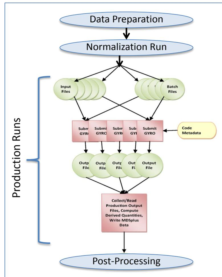
Workflow for preparing inputs and running a gyrokinetic simulation (M. Greenwald)
