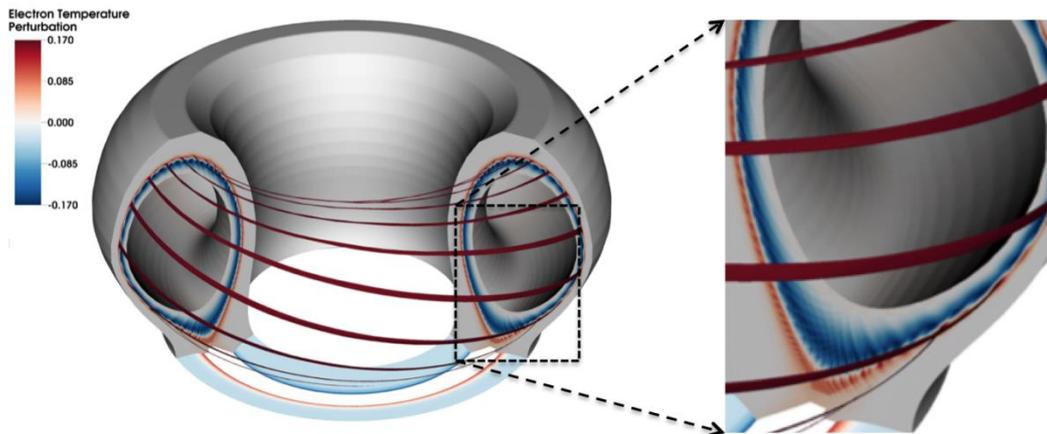
**BOUT++ simulation of 3D nonlinear ELM structure showing the perturbation to the electron temperature. Expanded view shows structure on both sides of the separatrix and in the divertor region with heat flux on the divertor plate.**
