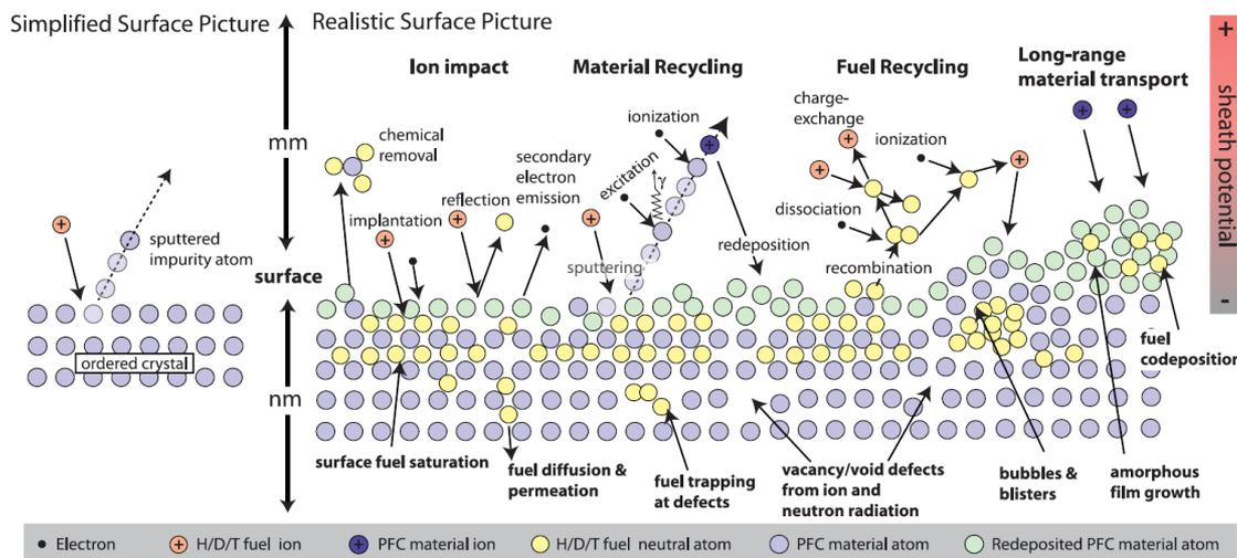
Comparison of a simplified plasma/surface model where only sputtering occurs (left) with a realistic model (right) where many types of interactions occur within the material during bombardment by a fusion plasma. Image courtesy of B. Wirth.
