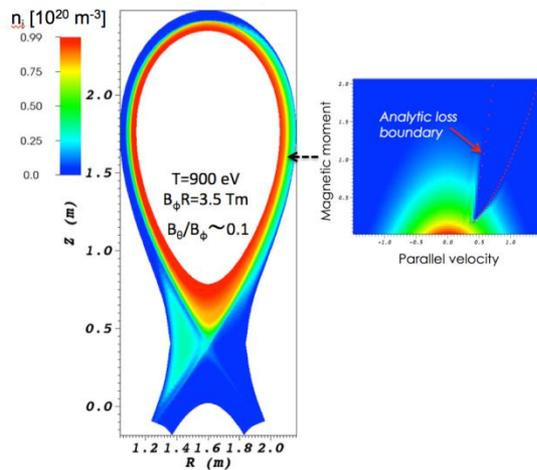
**COGENT 4D (2r,2v) kinetic simulation showing ion density and velocity-space loss cone for an initial uniform Maxwellian distribution function after 1.2 ms**
