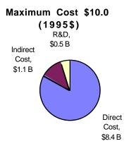
Direct construction costs include all components, systems structures, buildings, materials, and construction labor to construct the complete ITER facility that would operate during the basic performance phase. Indirect costs include project management, procurement, engineering, support of construction, and preoperational testing / startup. R&D includes the cost of R&D scheduled, but not performed during the EDA (~116M 1995\$) and R&D forecast as being needed during construction.
