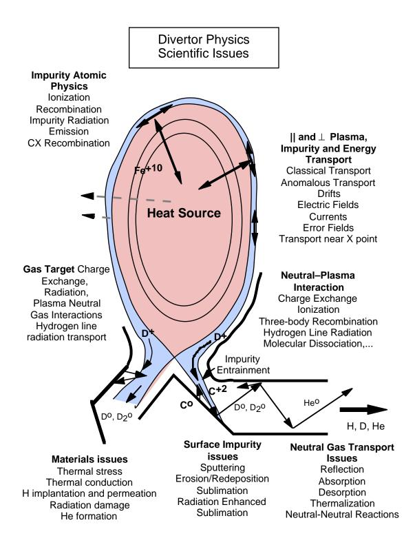
Figure II.D.1. Schematic illustration of divertor physics scientific issues
