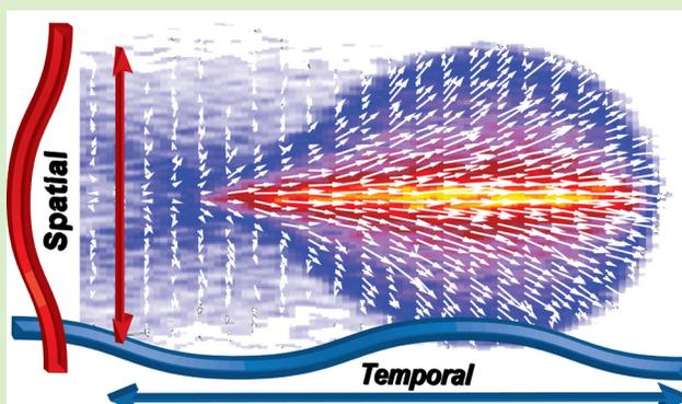
**Fig. 11.** Free-space propagating ultrashort electron pulse exhibiting collective and stochastic space charge dynamics. The electron pulse manipulation using longitudinal and transverse lenses to reconstruct electron six-dimensional phase space allows optimization of combined temporal, spatial, and spectroscopic resolution.
