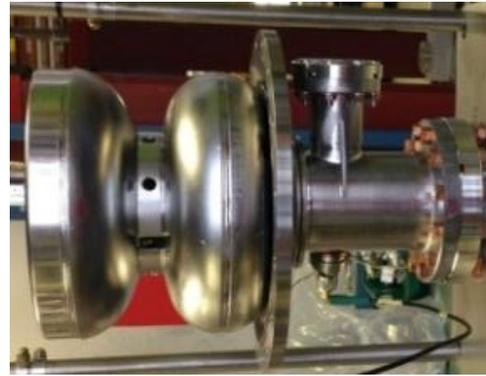
Figure 3-7: Drawing of the gun with superconducting cathode and picture of the cavity. Courtesy of DESY.
