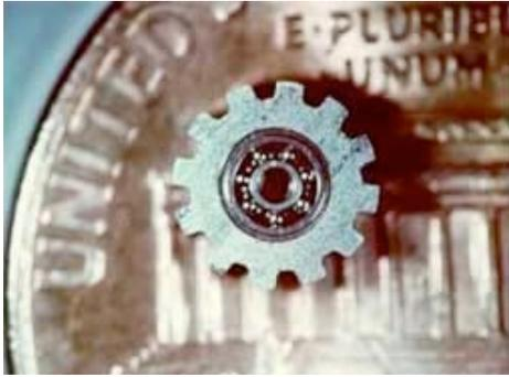
*LIGA-micromachined gear for a miniature electromagnetic motor.*
