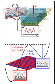
Figure 2. Top: schematic of Electrochemical X-ray reflectometry (XRR) cell developed at the Advanced Photon Source, Argonne National Lab. Bottom: XRR reveals that ionic liquids at charged graphene surface exhibit coexisting cationand anion-terminated patchy phases. (Uysal, et al., J. Phys. Condens. Matt. 2015, 27, 032101).
