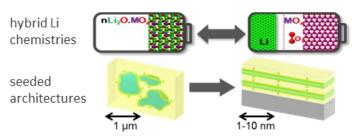
**Figure**: (Top) Schematic of interfacial structures and coatings to control secondary reactions at insertion electrodes interfaces. (Bottom) Directing chemical reactivity through the use of advanced architectures for conversion reactions and novel chemistries associated with hybrid Li<sup>+</sup>/Li-O reactions.
