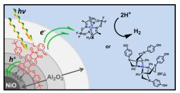
**Fig. 2.** Photocatalytic proton reduction by molecular catalysts in solution via electron transfer from a purpose-synthesized organic chromophore bound to a semiconductor surface.
