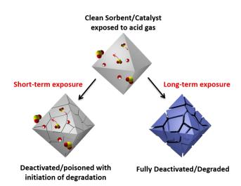
**Figure 1:** Changes induced in sorbents/catalysts upon short- and long-term exposure to acid gases. Materials are typically treated as passive in these environments, but can change dramatically upon exposure to  $SO_{x_1} NO_{x_2}$  and  $H_2S$ .
