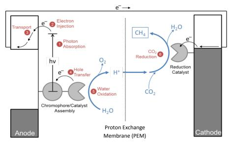
**Dye-Sensitized Photoelectrosynthesis Cell (DSPEC)**
