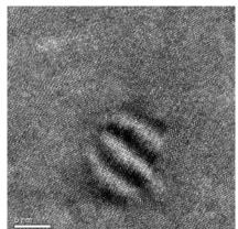
**Figure 1** High resolution TEM image showing spinodally decomposed regions in PbTe-16%PbS.
