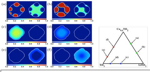
**Figure 1:** The concentration evolutions of Li (left side in each panel) and Cu (right side in each panel) during Li insertion ((a)-(b)), Li extraction ((c)-(d)), and Cu insertion ((e)-(f)). The corresponding points on the Gibbs ternary phase triangle are shown on the right.
