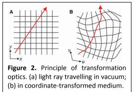
The RG-3 team addresses "*Transformation Optics for Photovoltaics*" will take a new approach to photovoltaic absorber design using optical focusing by transformation optics. Transformation optics provides a novel way to control the propagation of light using metamaterials - ordered artificial structures with features smaller than the wavelength.
