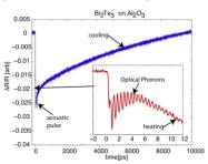
Figure 2: Ultrafast spectroscopy measurement of phonon dynamics
