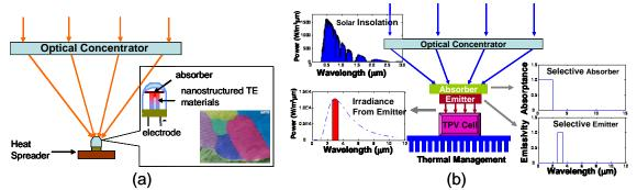
Figure 1 Solid-state solar-thermal energy conversion technologies to be pursued at the S<sup>3</sup>TEC Center (a) low-cost solar thermoelectric generators (STEGs) built from high performance nanostructured thermoelectric materials, and (b) high efficiency solar thermophovoltaics achieved via precision spectral control.
