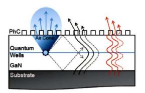
The objective of the Center's **Solid-State Lighting** research is to address the basic materials science and engineering required to achieve all semiconductorbased white-light sources with output greater than 300 lumens/watt, corresponding to greater than 80% wallplug efficiency. We intend to achieve these goals by: (1) pioneering the application of photonic-crystals to enhance the extraction efficiency of light-emitting
