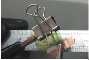
Figure 1. Transparent photovoltaic cell using graphene for both anode and cathode.
