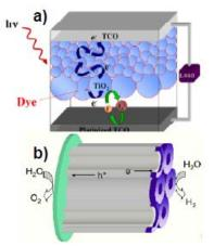
**Fig. 3. a)** DSSC based on electron injection into a wide bandgap, nanocrystalline, n-type semiconductor. **b)** *Compartmentalized* light-harvesting, catalytic oxidation, and catalytic reduction components function on a higharea, high-porosity, electrically conductive platform.
