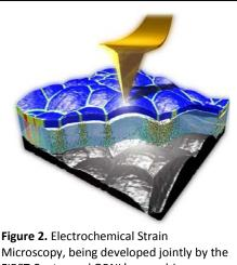
Microscopy, being developed jointly by the FIRST Center and ORNL's user-driven Center for Nanophase Materials Sciences, reveals the diffusional dynamics of lithium ions in working battery electrodes with nanometer resolution (Balke et al, *Nano Letters* **10**, 3420, 2010).
