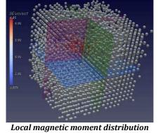
Local magnetic moment distribution at t=0.146 ps during a 500eV displacement cascade simulation of radiation damage in a 9826-atom BCC supercell of Fe
