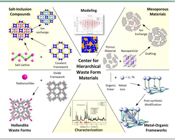
RESEARCH PLAN: Fundamental knowledge necessary to create new materials to safely sequester nuclear waste will be developed through the computationally-informed design of novel hierarchical materials, generating innovative chemical approaches and structure motifs through the use of advanced synthesis and characterization methods.
