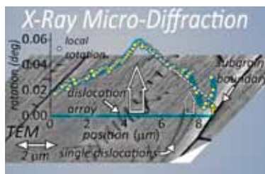
ABOVE: Submicron x-ray beams map the lattice rotations around dislocation lines identified in the underlying transmission electron microscope, or TEM, image. The dislocations at the large arrow collectively tilt the lattice. The isolated dislocations to the right (medium arrow) produce only localized rotations that generally cancel each other out. TOP: CDP doctoral student (right) characterizes with TEM a sample for CDP staff (left) to investigate with submicron x-ray microscopy.
