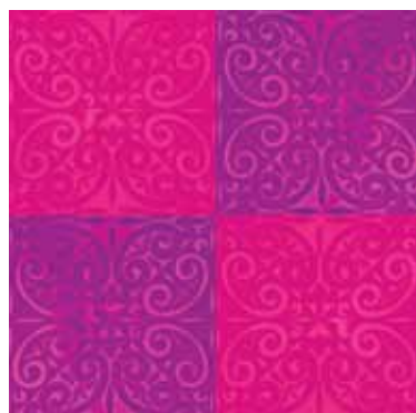
ABOVE: An example of an adaptive material in which magenta and violet colors reflect different modes of organization of nanoparticles irradiated with light of different wavelength. TOP: The first-ever micromachine powered by random motions of the surrounding bacteria. Bacterial motions are “rectified” by the geometry of the rotating gears.
