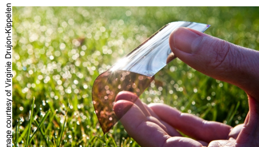
Image courtesy of Virginie Drujon-Kippelen Using polymers to develop new materials, EFRC researchers created the first completely plastic solar cell, where not just the cell itself but also its electrodes are made of plastic.
