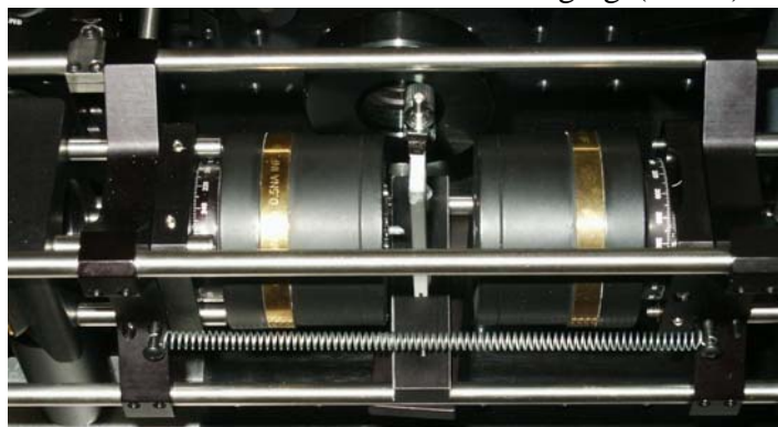
Fig. 1. The complete Kerr-gate assembly consisting of two Cassegrainian objectives, liquid Kerr medium (benzene), polarizers and the injection mirror.
