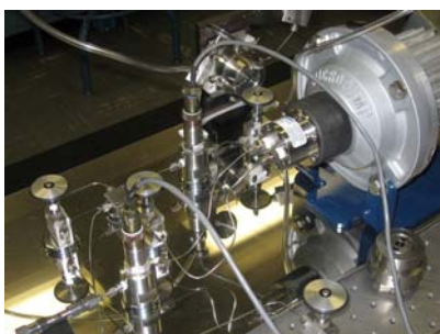
High-pressure apparatus for experiments in scCO 2 solution.
