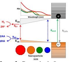
**Figure 2.** Energy level diagram showing the size dependent processes in CdTe-CaI
