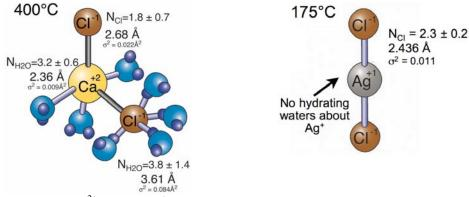
Figure 1. Schematics of the Ca<sup>2+</sup>/Cl<sup>-</sup> and Ag<sup>+</sup>/Cl<sup>-</sup> ion pairs at 400°C and 175°C, respectively.
