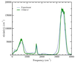
**Figure 2**. The IR spectra of liquid water obtained from classical simulations with the TTM3-F potential. The experimental results are also indicated.
