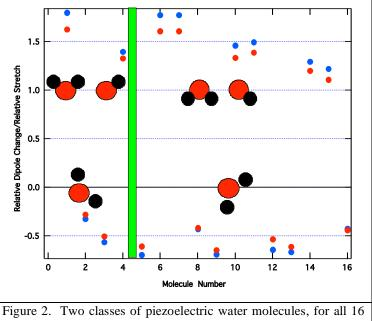
Figure 2. Two classes of piezoelectric water molecules, for all 16 molecules in the unit-cell used. Red/blue points are determined via squeezing/expanding the lattice. The first 4 molecules are updipole oriented, the rest down. Water molecules are shown that straddle the z-axis (top) or lay along it (bottom).
