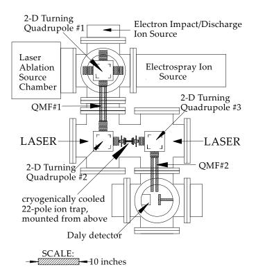
Figure 2. Design plan for the Utah ion trap photodissociation spectrometer.
