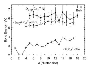
Figure 4. Comparison of the average cluster dinitride bond energies,  $D_0(\text{Co}_n^+-2\text{N})/2$  (open diamonds) with the average cluster nitride bond energies,  $D_0(\text{Co}_n^+-\text{N})$  (closed circles). The estimated bulk-phase value for N binding from Benziger (Ref. 10) to cobalt surfaces is shown to the right.  $D_0(\text{Co}_n^+-\text{Co})$  bond energies (Refs. 11 and 12) are indicated by open circles.
