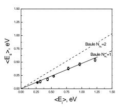
Figure 1. Comparison to the binarycollision limit. Final translational energy for scattered HCl: vibrationally elastic ( $v=2\rightarrow 2$ ) (open circles). All results shown here are for final J=5and  $T_s = 300$ K. The solid line shows the translational recoil expected from an zero impact-parameter elastic collision of an HCl molecule with an isolated Au atom. The dashed line shows results expected by doubling the effective mass of the Au atom.
