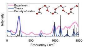
Fig. Inelastic neutron scattering from solid formic acid in the  $\beta_1$  form.
