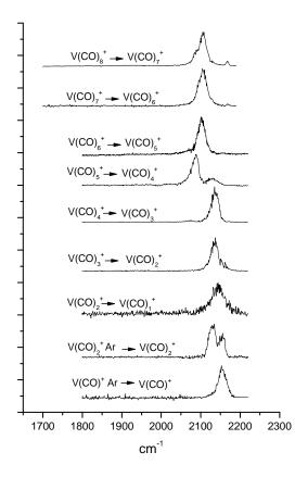
Figure 1. The IR spectra of  $V^+(CO)_n$  complexes measured with mass-selected photodissociation.
