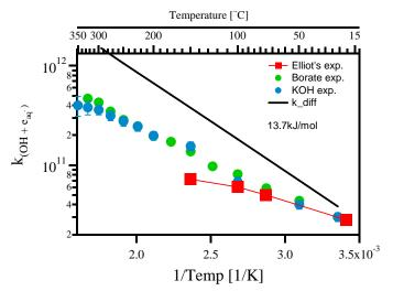
**Figure 1** – Arrhenius plot for reaction of  $e_{aq}^-$  with OH. New results are compared with literature values of Elliot and an estimate of the diffusion limit k\_diff.
