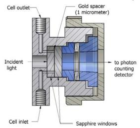
**Figure 1** – Flow cell designed for optical absorption measurements in supercritical fluids.
