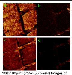
100x100µm<sup>2</sup> (256x256 pixels) Images of Cu grid embedded in In. (a) and (b) are PI images of In and Cu, respectively. (c) and (d) are SIMS images.
