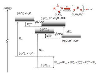
**Figure 2.** Illustration of the thermodynamic cycle, including relaxation, used to obtain monomer dissociation energies for small neutral water clusters from their measured vertical ionization energies.
