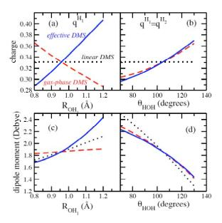
Figure 1. Atomic charges and total dipole moment for water monomer. Dotted lines: linear DMS (constant charges). Dashed lines: non-linear DMS (geometry dependent charges). Solid lines: non-linear "effective" DMS.
