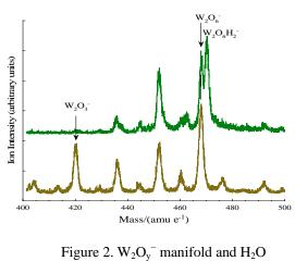
Figure 2.  $W_2O_y$  manifold and  $H_2O$  reaction products.
