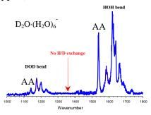
**Figure 1.** Ar predissociation spectrum of  $D_2O \cdot (H_2O)_6 \cdot Ar_6$  product ions from condensation of  $D_2O$ molecules onto the  $(H_2O)_6 \cdot Ar_{12}$  parent cluster, in the region of the bending fundamentals of the  $H_2O$ ,  $D_2O$  and HOD molecules. These data indicate that the  $D_2O$  molecule can displace the  $H_2O$  molecule at the AA binding site for the excess electron.
