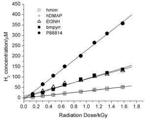
**Figure 2** – Comparative plot of H2 yields depending on radiation dose applied to five different RTILs
