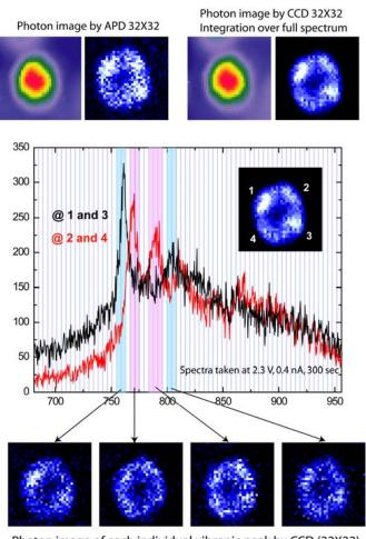
Photon image of each individual vibronic peak by CCD (32X32)
