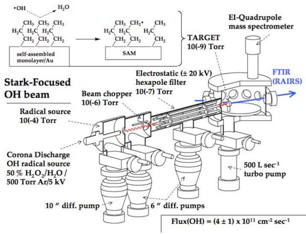
Dosing of the film with OH for 1 min. results in degradation of both  $v_a(CH_3)$  and  $v_s(CH_3)$  signals; by 10 min. both signals are largely destroyed while the CH<sub>2</sub> signals are still intact. The RAIRS spectra are shown in the Fig. below. During a 10 min. interval the alkyl SAM which is mounted on a 1 cm<sup>2</sup> target is dosed with 10 x 60 x (4 x 10<sup>11</sup>) or 2 x 10<sup>14</sup> OH radicals. This is roughly 50% of a
