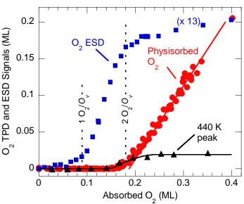
Fig. 1. O<sub>2</sub> TPD and ESD signals versus O<sub>2</sub> coverage.
