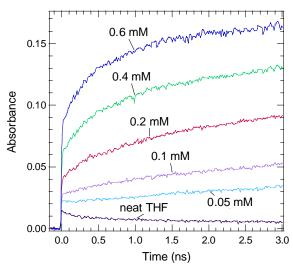
step is due to capture of pre-solvated ("dry") electrons. The step furthermore corresponds to  $\sim$ 50% of the total number of electrons captured at longer times, which is a huge advantage for measuring fast electron mobility on the wires by transport to attached end caps.
