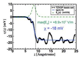
**Figure 1.** The TZV2P electrostatic potential  $\varphi(z)$  data (black circles) along with a tanh fit (smooth solid blue curve) to the  $\varphi(z)$  data and the corresponding interfacial electric field  $E_z(z)$  (dashed green curve). The Gibbs dividing surface is located at z = 9 Å (vertical dotted line).
