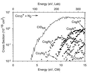
Figure 3. Reaction of  $\text{Co}_{10}^+$  with N<sub>2</sub> showing cross sections for dinitride (open symbols), mononitride (closed symbols), and the total CID products (solid line).
