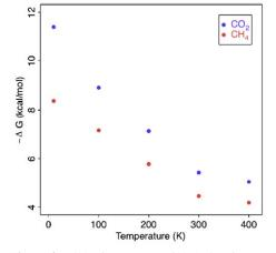
**Figure 2.** Gibbs free energy of inclusion for a single  $CO_2$  or  $CH_4$  molecule in TBC4 at various temperatures.
