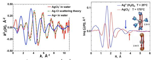
Figure 2. XAFS  $k^2$ -weighted  $\chi(k)$  and  $\text{Im}[\tilde{\chi}(R)]$  plots for hydrated and ion-paired Ag<sup>+</sup> showing the significant photoelectron multiple scattering features used to establish the first-shell symmetry.
