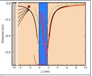
**Figure 1** The blue shaded region shows 1.8 nm water film, within a 3-methylpentane film (salmon). The measured solvation chemical potential for a single ion approaching the water film is the heavy black solid line. The red curves are Born calculations for  $5\text{\AA} = r_b$ ,  $\epsilon_1=1.9$ ,  $\epsilon_2=100$ , and water films 0.15, 0.3, 0.45. 0.6, 1.8, and 3.0 nm (7.1 ML) thick. Green curve is Born model for a 1.8 nm water film with  $\epsilon_2=5$ .
