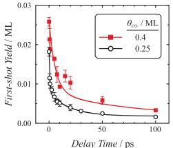
**FIG. 1.** Two-pulse correlation measurements of the ejected  $CO_2$  photoproduct from CO+O/Pd(111) at initial CO coverages of 0.25 ML (circles) and 0.4 ML (squares) deposited on the O-(2×2)/Pd(111) (0.25 ML O) surface.
