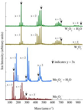
Figure 1. Comparison of water reactions with  $Mo_xO_y^-$  and  $W_xO_y^-$ .
