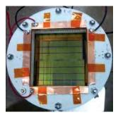
Fig. 3: Four inch phased array antenna THz source, developed by Rex Garland. The tiles are 1 cm interdigitated conductors with 10 micron spacings on a polished GaAs substrate.
