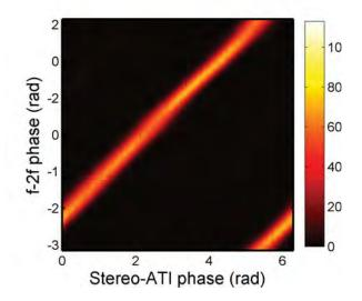
Figure 1: The distribution of synchronized measurements of the CEP using a single-shot f-2f spectrometer and a stereo ATI phase meter. A total of six million laser shots were monitored. The standard deviation of the difference between the two phases was 220 mrad.
