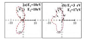
**Fig.1:** CADs in beV<sup>-1</sup> sr<sup>-2</sup> for emission of one electron (black arrows) along the linearly polarized electric field of a 99 eV,  $10^{14}$  W/cm<sup>2</sup>, 0.5 fs XUV pulse. E<sub>1</sub> and E<sub>2</sub> are the approximate asymptotic energies of the emitted electrons. The black dots with error bars are experimental results [R1]. The red dashed lines are our calculated results. (a) Equal energy sharing. (b) Unequal energy sharing.
