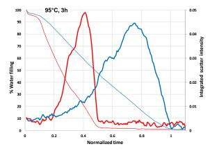
**Figure 3:** Water content in CNTs (thin lines, left scale) and x-ray scatter signal (heavy lines, right scale) of wet nanotubes normalized by that of dry nanotubes. The signals form the heat-treated CNTs are plotted in red and from the untreated CNTS in blue.
