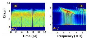
**Fig.3:** (a) Probability density and (b) corresponding power (or QB) spectrum (logarithmic color scale) for the external-field-free propagation of nuclear vibrational wave packets in the  ${}^{2}\Sigma_{u}^{+}$  adiabatic electronic state of  $Ar_{2}^{+}$ .
