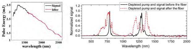
Figure 2: a) Energy per pulse in the signal (black) and idler (red) out of the HE-OPA as a function of wavelength. The maximum total energy is 6 mJ (signal + idler), b) Simultaneous broadening of the signal and depleted pump after SPM. Pulse durations, as measured by a SHG-FROG are 6.5 fs for the depleted pump and 15 fs for the signal (1300 nm).
