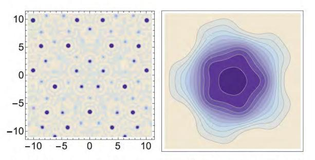
Figure 2: Phase reconstruction of AlCuRh quasicrystal diffraction data. *Left:* Electron density in a 5-fold plane of the decagonal quasicrystal. The very darkest and weakest spots correspond to Rh and Al atoms respectively. Intermediate density spots are Cu and Cu/Al mixed occupancy positions. *Right:* Phase reconstruction of the "superspace atomic surface", a structure that encodes site occupancy in the quasicrystal more compactly than non-periodic density maps.
