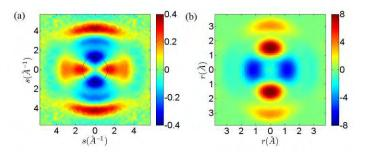
Figure 2. a) Diffraction pattern of aligned CS<sub>2</sub> molecules. b) Fourier Transform (FT) of the diffraction pattern. The structure and angular distribution can be extracted from the FT. The bright spots in the vertical direction correspond to the C-S and S-S distance (1.55Å and 3.1Å, respectively).
