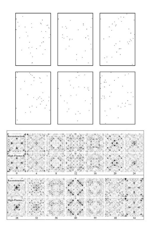
Figure 1: *Top*: Six diffraction data frames of a crystal in one orientation. At these ultra-low-signal levels there are no discernible Bragg peaks to help orient the frames. *Bottom*: Comparison of Patterson maps derived from the true 3D intensity and the intensity reconstructed from 290,000 low-signal data frames.
