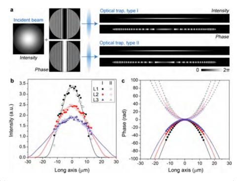
Figure 4: (a) Optical beam, phase profiles programmed onto a 2D spatial light modulator (SLM) and the resulting calculated intensity and phase profiles. (b) Measurements of the intensity and phase profiles of line traps of various widths. Both + and - phase profiles (that have the same intensity profiles) are generated and measured using a Shack-Hartmann wavefront sensor.
