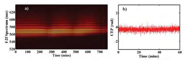
Figure 1: a) Single shot f-2f spectra measuring the CEP after the second stage amplification of HITS. RMS deviations in the CEP over the 750 minutes is 320 mrad. b) Single shot phase calculated from the first 60 minutes of the spectrum in a). RMS deviation of the CEP is 220 mrad over this hour.
