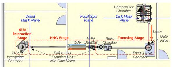
Fig. 2. Top view schematic of the new XUV beamline.
