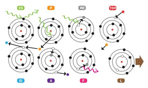
Figure 3: Primary and secondary electronic processes important to consider in interactions of XFEL pulses with matter: elastic x-ray scattering (ES), photoionization (P), resonant excitation (RE), threebody electron-ion recombination (TBR), electron-impact ionization (EI), Auger decay (A), fluorescence (F), and lattice dynamics (L).
