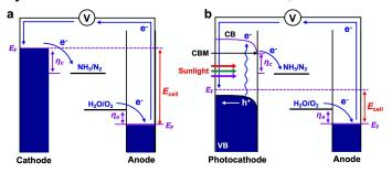
**Scheme 1.** Schematic comparison of (a) electrochemical and (b) photoelectrochemical N<sub>2</sub> reduction, illustrating why the use of a photocathode can decrease the overall cell voltage needed to operate the N<sub>2</sub> reduction cell (E<sub>cell</sub>: voltage required to operate the cell, E<sub>F</sub>: Fermi level, CB: conduction band, VB: valence band, CBM: conduction band minimum,  $\eta_c$ : cathodic overpotential,  $\eta_a$ : anodic overpotential).
