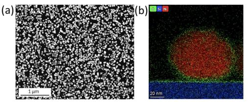
Figure 1: (a) SEM micrograph showing electrodeposited Ni with average diameter of 70 nm on top of a Si substrate. (b) EDS/STEM cross-sectional micrograph showing an individual Ni nanoparticle with an oxide layer at the Ni/Si interface.
