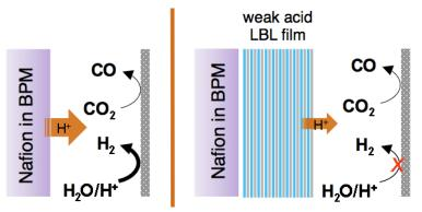
Fig. 1. Layer-by-layer assembly of a weakly acidic cation exchange layer modulates the local pH at the catalyst surface in a bipolar membrane based  $CO_2$  electrolysis cell. Higher local pH improves the conversion efficiency of  $CO_2$  to CO by suppressing the competing hydrogen evolution reaction. (Z. Yan et al., *Nat. Chem.* 13, 33–40 (2021)).
