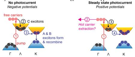
Figure 1. Fundamental processes in a photoelectrochemical cell made from ML MoS<sub>2</sub>.
