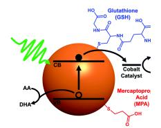
**Figure 1:** System for photochemical H<sub>2</sub> production using a cobalt catalyst.
