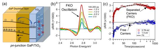
**Figure 1.** (a) Schematic diagram illustrating the GaP/TiO<sub>2</sub> photoelectrode. (b) Potential-dependent FKO oscillation strength and (b) corresponding free carrier and separated carrier kinetics.
