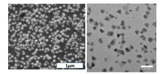
Figure 1 SEM image of crystal InSb QDs on  $SnO_2$  with 1000 cycles of trimethyl indium and trisdimethylamido antimony followed by 120 cycles of TiO<sub>2</sub> deposition (left). InSb nanocrystals deposited directly on a TEM grid. (right)
