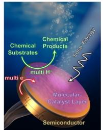
**Figure 1.** Schematic illustration of a molecular catalyst-modified photoelectrode. Figure adapted from cover image of reference 2.
