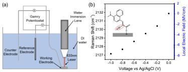
**Figure 2.** (a) Schematic diagram illustrating our photoelectrochemical measurement setup with *in situ* Raman spectroscopy. (b) Raman shift of the nitrile stretch measured as a function of the applied electrochemical potential.
