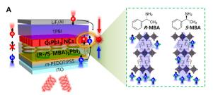
**Figure 1.** Spin-LED consisting of a chiral-metal halide hole-transport layer and a non-chiral metal-halide light emitting layer.
