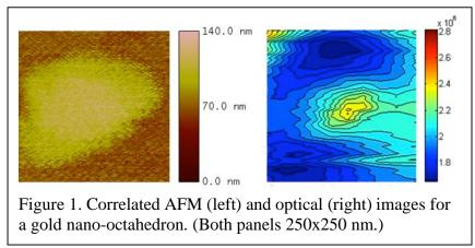
significantly beyond the diffraction limit and is smaller than the AFM image of the overall particle. The optical image also exhibits interference fringes at a larger scale. The apex image was created by collecting light during the entire oscillation period of the scanning tip; this effect averages the enhancement factor, that only is large when the tip is very close to the particle. We will use a gated CCD camera to eliminate this problem.
