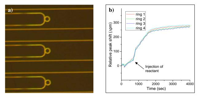
**Figure 1.** (a) An optical micrograph of three Si photonic ring resonators that are optically interrogated by adjacent waveguides. (b) The addition reaction of a  $\sim$ 150 amu molecule covalently linking to an organic thin film can be monitored in real time by measuring the frequency shift in the cavity modes of a ring resonator.
