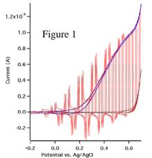
that previous studies had indicated. We have successfully synthesized Si-doped hematite films by chemical vapor deposition. These films are highly photoactive, achieving photocurrents for water oxidation that are comparable to the best films made by others. An example of a chopped-light photocurrent characterization experiment is given in Figure 1.
