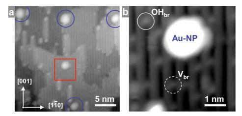
Figure 1. Cryogenic STM on small Au nanoparticles on rutile  $TiO_2(110)$ . a) Overview scan, showing several Au particles with lateral dimensions of 2 – 3 nm and height of ~ 0.5 nm (blue circles). b) High-magnification view of the area marked red in a). Circles mark  $TiO_2(110)$  surface defects, whose nature (OH<sub>br</sub> – bridging hydroxyl; V<sub>br</sub> – bridging oxygen vacancy) was directly identified by manipulation techniques.
