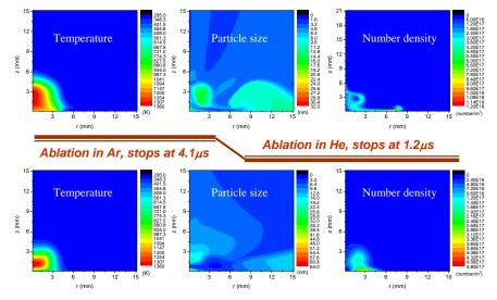
Figure 1. The simulated temperature, particle size, and number density distributions for ablation in argon and helium
