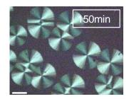
Figure 2. Optical micrograph of spherulites formed in a 240 nm thick PEGMEMA film at 23 °C. The samples are viewed using crossed polarizers, and the scale bar represents 100 µm.
