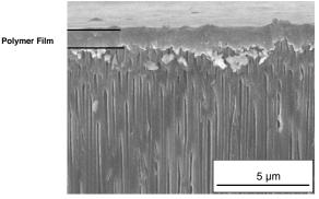
Figure 1. Composite membrane formed by polymerization of PEGMEMA (n=22-23) from porous alumina.
