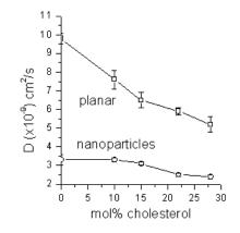
Figure 2. The diffusion coefficient of labelled lipids in planar bilayers vs. bilayers supported on silica nanoparticles.
