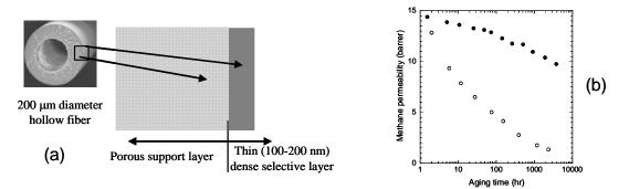
Figure 1.(a) Typical asymmetric hollow fiber membrane with ultrathin selective layer supported on an open cell porous layer, which also has untrafine submicron porous features; (b) Methane permeabilities in 6FDA-DAM:DABA (2:1) crosslinkable films of 49  $\mu$ m thickness (•) and 600 nm thickness (•).
