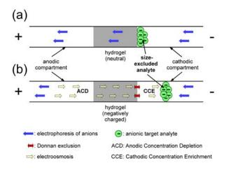
Figure 1.Concentration enrichment scheme with (a) neutral, and (b) anionic hydrogel membrane.
