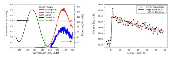
**Figure 3.** A Kerr-gated spectrum and the fluorescence decay of the 4-dimethylamino-4'-nitrostilbene (DNS) in tetrahydrofuran.
