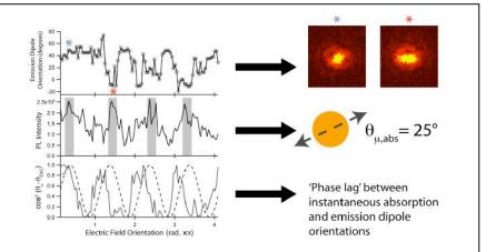
**Figure 1.** (Left) Comparison of emission moment orientation (top) and polarization anisotropy (middle) from a single 12-nm CdSe-oPV nanostructure. (Right) Defocused fluorescence images (filtered to include only the CdSe emission) show linear polarized emission with dipole orientation correlated with excitation polarization, with a phase-lag of  $\approx 25^{\circ}$  between the absorption and emission moments.
