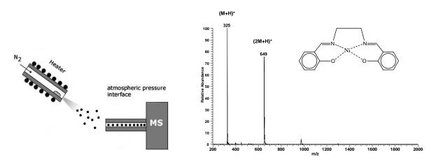
Figure 2: (left) Schematic of the APTDI process; (right) APTDI spectrum obtained from a Ni(salen) sample
