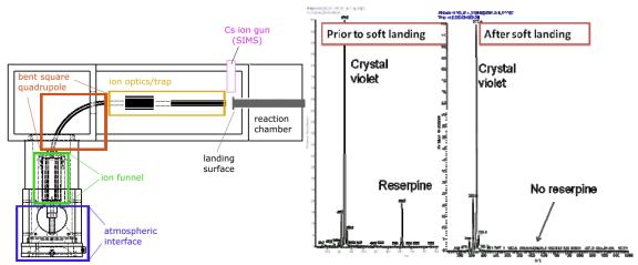
**Figure1:** (left) Schematic of our soft landing instrument; (right) Nanospray spectrum obtained after rinsing the soft landed surface. Crystal violet (m/z 371) was mass selected from reserpine (m/z 610) using an RIT in RF/DC mode, as evidenced by the lack of a reserpine peak
