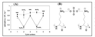
**Figure 2.** (A) The  $|\Delta D/(\Delta f/n)|$  ratio of an adsorbed layer obtained after washing with DI water. Change in frequency was normalized with the overtone number (*n*=7). Exchange of Br<sup>-1</sup> with SO<sub>4</sub><sup>-2</sup> ions resulted in a decrease in the  $|\Delta D/(\Delta f/n)|$  ratio while the reverse increased the  $|\Delta D/(\Delta f/n)|$  ratio almost back to its initial value. The decrease in
