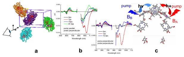
Figure 1. Ultrafast transient absorption measurements in reaction center single crystals. (a) Reaction center orientation in the  $P2_12_12_1$  crystals; (b) transient spectra using parallel and perpendicular 810 nm pump orientations, fixed perpendicular probe orientation; (c) cofactor specific excited-state pathways.
