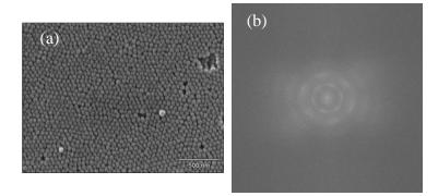
**Figure 1.** (a) SEM of array of  $50 (\pm 6)$  nm diameter silica nanoparticles assembled onto silicon substrate with thermally-grown silica overlayer; (b) FFT of SEM image .
