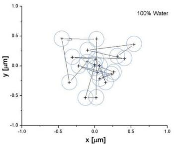
Figure 1. Diffusional trajectory of DiI on C18-modified silica surface in contact with water (30 ms time steps).
