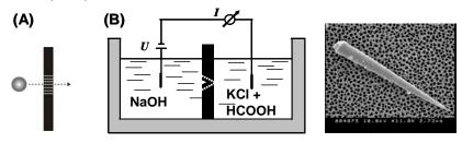
**Figure 1.** Preparation of PET membranes with single conical pores. (A) Irradiation of a polymer foil with a single swift heavy ion; (B) Experimental setup used for one-sided etching, which leads to the formation of conical pores; (C) 'Negative' of a conical nanopore obtained by electroless plating with gold of a single conical nanopore in PET.
