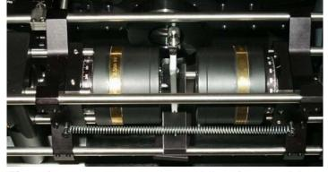
**Figure 1**. The Kerr-gate assembly consisting of Cassegrainian objectives, Kerr medium, polarizers and the injection mirror.
