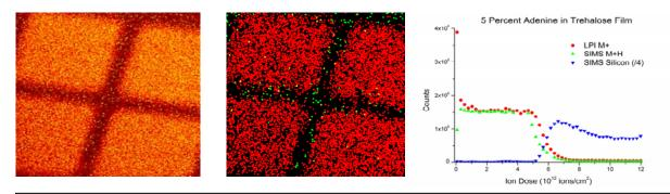
Figure 2. (left) Total laser-induced ion image taken over a  $200x200 \,\mu\text{m}^2$  field of view. (middle) Mass selected image; adenine (m/z 135) in red and silicon (m/z 28) in green. (right) Molecular depth profile of 5 percent adenine in a trehalose film; laser-induced in red, SIMS in green, substrate in blue.
