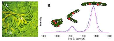
**Figure 3**: (A) Far-field fluorescence image of an annealed 6OPV film (i) a region exhibiting ribbon-like structure (ii) a region exhibiting amorphous structure(B) Arrival time distribution taken from a laser desorbed film of 5OPV
