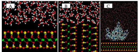
Figure 1. MDS snapshots of water molecules at talc basal plane (A), talc edge (B) surfaces, and adsorbed DTAB molecules at the talc basal plane surface(C). (Red-oxygen atoms, white-hydrogen atoms, blue-nitrogen atoms, purple-bromide atoms, yellow-silicon atoms, green-magnesium atoms, blue-nitrogen atoms, and light blue-carbon atoms.)
