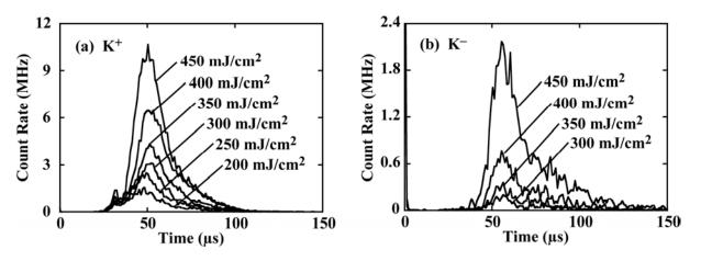
Figure 1. Time of flight signals of the positive (left) and negative (right) K ions from KCl for several fluences at 248 nm.
