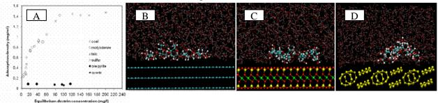
Figure 2. Dextrin adsorption isotherm (A) and MDS snapshots of "dextrin" adsorption states at graphite basal plane (B), talc basal plane (C), and sulphur (D) surfaces (Red-oxygen atoms, white-hydrogen atoms, blue-nitrogen atoms, purplebromide atoms, yellow-silicon/sulfur atoms, green-magnesium atoms, and light blue-carbon atoms.)
