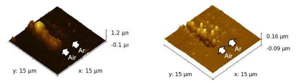
Figure 3. Nano patterns with in air and argon (a) before dipping in HF solution (b) after dipping in HF solution
