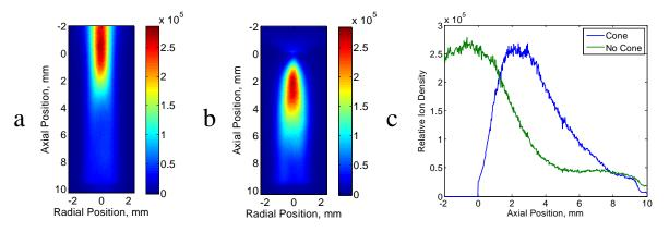
Figure 2. (a) Relative barium ion densities in the absence of a sampling cone. (b) Relative barium ion densities in the presence of a sampling cone. (c) Centerline traces (r = 0) from parts a and b.
