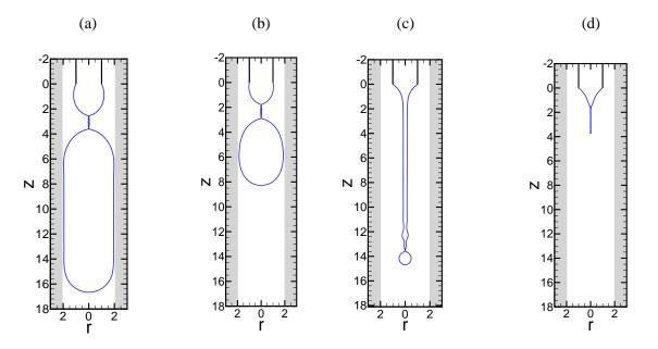
Figure 1. Focusing a liquid emerging from an inner tube by subjecting it to the flow of a faster moving surrounding liquid that is flowing in a concentric tube of larger radius. Here  $Q_r$  varies as (a) 0.1, (b) 10, (c) 30, and (d) 35.
