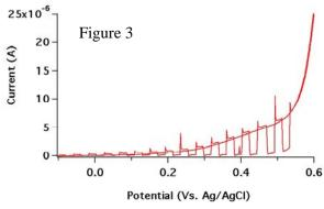
generated by a hematite-coated Pt/Ir tip in blue laser light. We are able to achieve  $\sim 5 \ \mu A$ currents in blue laser light.
