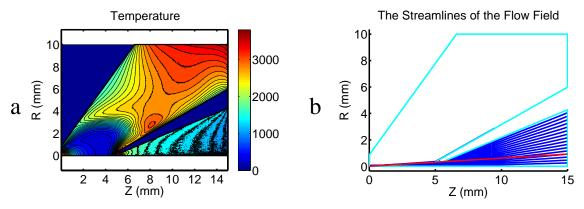
Figure 1. (a) Temperature contours in the first vacuum stage of an ICP-MS showing the formation of a secondary shock at the tip of the skimmer cone. (b) Flow streamlines showing secondary expansion downstream from the skimmer tip.
