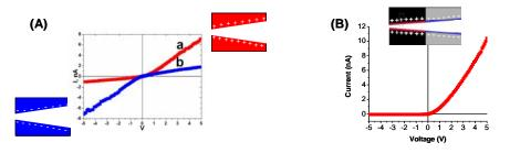
**Figure 2.** Transport properties of single conical nanopores with (A) homogeneous surface charges as shown in the insets, and (B) with surface pattern. The current-voltage curves were recorded in 0.1 M KCl, pH 5.5. Small opening of these pores was smaller than 5 nm [Ref. 2].
