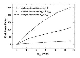
Figure 2. Steady-state enrichment factors as a function of the applied electrical field strength ( $E_{ext}$ ) for uncharged ( $c_{fix} = 0$ ), weakly charged ( $c_{fix} = 0.1c_{res}$ ), and highly charged ( $c_{fix} = c_{res}$ ) membranes.
