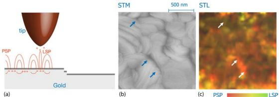
Figure 1. Imaging of plasmon modes on a Gold substrate covered with a 1,6-hexane-dithiol selfassembled monolayer. (a) Illustration of the two possible modes. (b) STM image of the imaged area (c) simultaneously collected tunnelling luminescence image. The color indicates which mode is active where.
