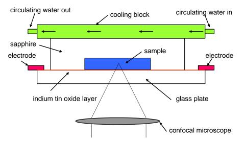
Figure 1. Schematic drawing of the cell used for generating a linear thermal gradient. The hot surface is provided by the electrically heated indium tin oxide coating on a piece of glass; a cold surface is maintained by circulating water through a cooling block. Current is fed from a power supply to the electrodes.
