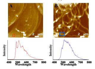
**Figure 4**: NSOM images and spectra from annealed 6OPV films (A) a "sheet-like" region with fluorescence spectrum from boxed region (B) a "ribbon-like" region with fluorescence spectrum from boxed region
