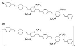
Fig. 1. Structures of OPV  $(6R\text{-}4OC_8H_{17})\,(a)$  and TOPV  $(T\text{-}6R\text{-}4OC_8H_{17})\,(b).$
