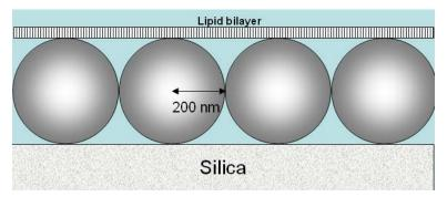
Figure 1. Silica nanoparticles of 200 nm in radius form an ordered monolayer on silica. The lipid bilayer is suspended above the nanoparticles.
