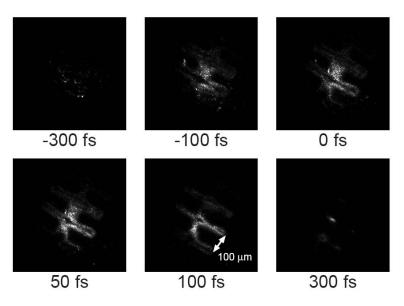
**Figure 4.** Time resolved reflection image of an etched glass surface. The instrumental response function is 130 fs.
