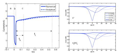
Figure 1. (*Left*) Ionic current vs time when the system is positively biased. (a) current during the rest stage, (b) current during the injection stage, and (c) current during the recovery stage. (*Right*) Ion concentration along the central line of the source channel during the recovery stage. Note that the recovery stage starts from t = 25 ms. (*Top*) cation concentration. (*Bottom*) anion concentration.
