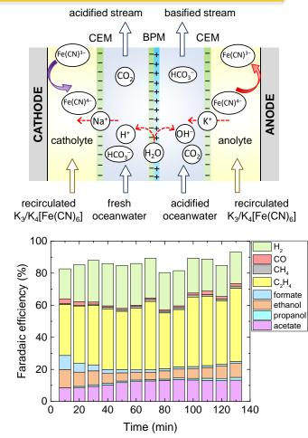
Schematic illustration of the BPM electrodialysis cell, and gas/liquid product distribution of converted  $CO_2$  from ocean water..
