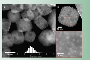
Electron micrographs of Pt NPs with an average size of  $2.0 \pm 0.5$  nm, deposited by ALD on SrTiO<sub>3</sub> nanocuboids
