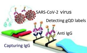
Lateral Flow Assays (LFAs) for immune response. Demonstration of a LFA platform for inexpensive yet highsensitivity/high-reliability rapid diagnostics for COVID virus and antibodies. (CINT)
