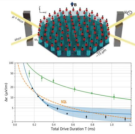
A) Beryllium ions (red dots) confined within a Penning trap. The valence electron spin (black arrows) of the ions realizes a collective spin that serves as the measurement device.
