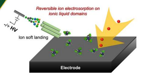
Dissolved ILCs are ionized by electrospray ionization and then deposited onto the electrode surfaces. Once adsorbed, the ILCs reduce the amount of energy needed for other ions from solution to adsorb and separate on the electrode.
