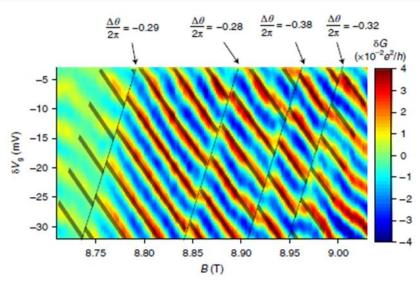
Map of the conductance (color scale) versus magnetic field (B) and gate voltage in a 2D electronic device. Each dashed line denotes a jump in the phase of the quantum-mechanical wave of the system, corresponding to a rotation of a fraction (1/3) of  $2\pi$ . This fractional rotation is the smoking gun for the presence of exotic particle-like objects called anyons.
