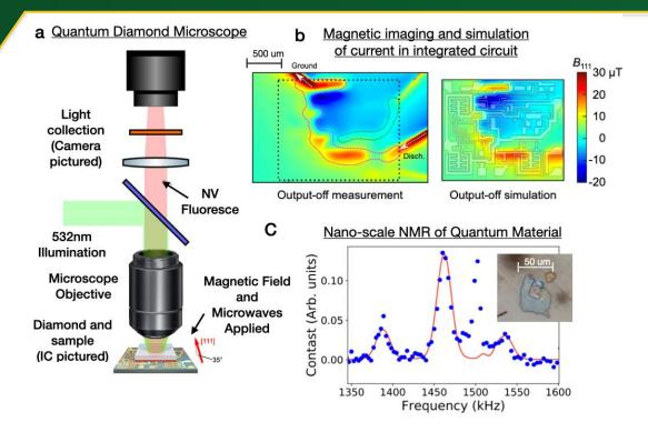
(a) Cartoon of Quantum Diamond Microscope experimental implementation at CINT. (b) Widefield quantum-sensed magnetic fields from integrated circuit and complete modeling of device.[2] (c) NMR spectrum for <sup>11</sup>B in hBN as detected by nitrogen vacancy ensembles. (inset) 100nm thick hBN flake on nitrogen vacancy rich diamond. [3]
