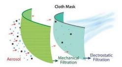
Schematic showing filtration of aerosol particles using a combination of mechanical and electrostatic filtration from a combination of fabrics. The study found that fabrics with a tight weave and low porosity, such as those found in cotton sheets with high thread count, performed well. (Image courtesy of American Chemical Society)
