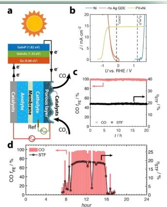
(a) Wire connection between the triple junction PV and GDE cell. (b) *J-U* characteristic of Ni anode, photovoltaic with Ni anode, and Ag-NP gas diffusion cathode under 1 Sun. (c) The CO Faradaic efficiency and solar to fuel efficiency over the 20 h duration in lab under 1 Sun. (d) The CO Faradaic efficiency and solar to fuel efficiency for a 24h day under outdoor illumination in Pasadena, CA.
