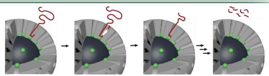
Steps in the processive polymer deconstruction mechanism: (a) PE adsorption into a pore, (b) cleavage of a C-C bond via hydrogenolysis, desorption of the short hydrocarbon fragment, and repositioning of the adsorbed chain, (c) repeated cleavage, product release, and chain reorientation to convert the entire strand into a uniform distribution of shorter chains.
