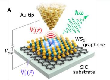
Scanning Tunneling Luminescence photon counts
