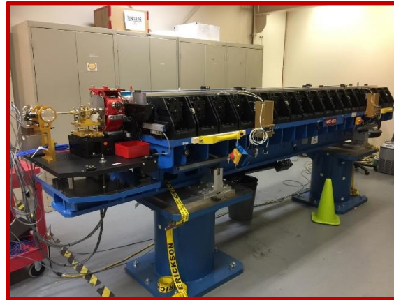
13 of 32 hard x-ray undulators were delivered
