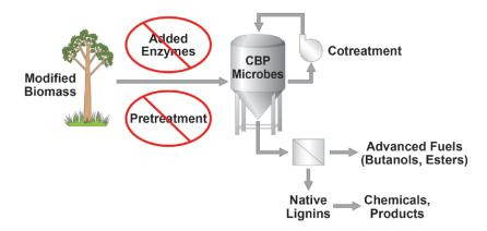
Consolidated Bioprocessing (CBP) and **Cotreatment Para**digm. CBP combines the three biologically mediated steps for biomass processing (cellulase production, enzymatic hydrolysis, and microbial fermentation) into a single operation, thereby eliminating the need for added enzymes and pretreatment. **CBP** implementation requires microbes that can produce a functional cellulase system while generating advanced fuels at high yields and concentrations. [ORNL]
