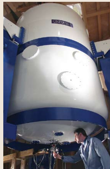
EMSL's 900-MHz Nuclear Magnetic Resonance Spectrometer. This instrument is used to provide atom-by-atom, three-dimensional views of protein complexes and other molecular structures.
