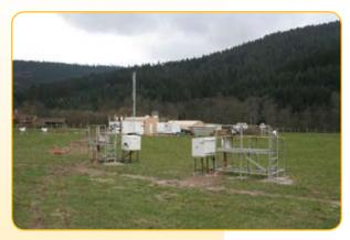
**Continuous Atmospheric Data for Researchers Worldwide.** Each ACRF site includes a broad array of instruments for observing the surface radiation balance and the atmospheric properties that drive that balance.
