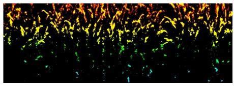
Side-profile of a row of mature corn (10 ft tall) using downward-facing LiDAR (color indicates height), showing the high resolution and canopy penetration that Blue River's drone LiDAR data provide. Extracted from the full field above.
