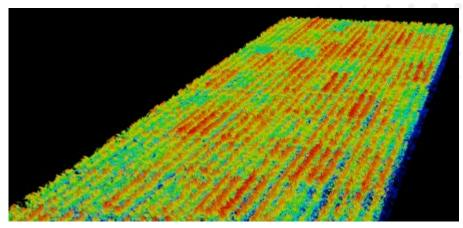
Corn breeding plots in a drought stress trial. Color is height measured by LiDAR.
