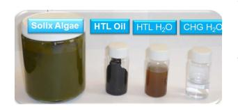
**Whole algae HTL Development:** Continuous bench-scale liquefaction, separations, upgrading, and carbon recovery from waste-water for 10 unique algal feedstocks
