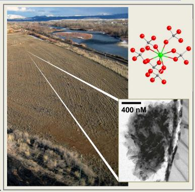
Mobile uranium(VI) in the contaminated DOE-Rifle, CO aquifer (above) is reduced to relatively immobile U(IV) by nano-phase iron sulfides precipitated on bacterial biomass (lower right). Upper right: A structural analog for U(IV) complexed to biopolymers.
