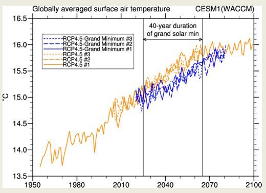
Time series of globally averaged surface air temperature anomalies (°C) relative to the 1986-2005 reference period for the CESM1(WACCM) standard RCP4.5 simulations (orange lines) and the grand solar minimum experiment (blue lines). The duration of the grand solar minimum experiment is indicated from 2025-2065.
