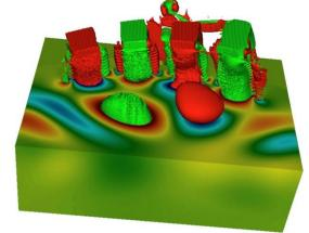
Simulation of the Alcator C-Mod Field Aligned Antenna in pimode. The left plot shows fast wave propagation from the antenna for high-edge density. If slow waves are present, their field amplitudes can be high and can contribute to both the amplitude of the radio frequency sheath voltage and to parasitic power losses in the edge plasma.
