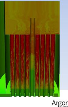
(Right) Temperature distribution in the MASLWR core computed using Nek5000 (frozen velocity)
