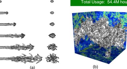
(a) Snapshots of EHD enhanced kerosene atomization simulation. Time varies from t=0.0 s (top) to t=0.0005 s (bottom). (b) Topology of liquid gas interface interacting with turbulence. *Image Credit: Oliver Desjardins, Cornell University*
