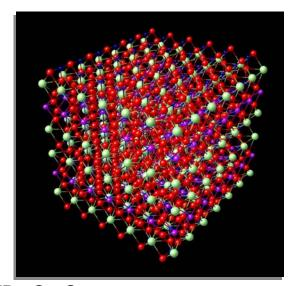
Model of a YBa<sub>2</sub>Cu<sub>3</sub>O<sub>7</sub> high-temperature superconductor crystal
