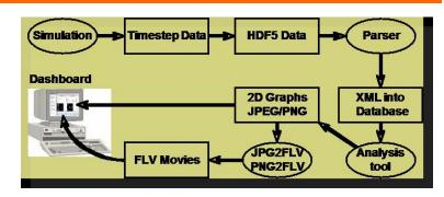
Monitoring workflow schematic using Kepler workflow system
