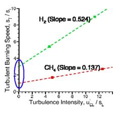
Quantifying dependence of burning rate on turbulence intensity for different fuels, with substantial impact on engineering design.
