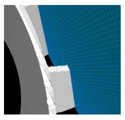
Low-swirl injector for gas turbine. **Left:** surface description from embedded boundary grid generator. **Right**: blowup showing intersection of the grid with the vanes.
