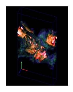
Hydroxyl radical in a turbulent jet flame
