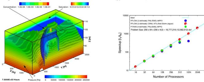
Sample computation using the PETSc powered PFLOTRAN subsurface flow simulator and its parallel performance on the DOE leadership-class Cray XT3 system
