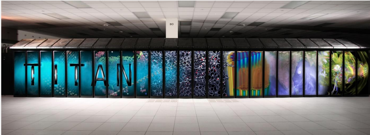
Figure X: Titan. By upgrading its Jaguar machine and installing NVIDIA GPUs, ORNL created Titan, which reclaimed the No. 1 position on the TOP500 List.
