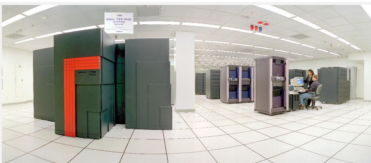
Fig. X: T3E 900. NERSC's Cray T3E-900 provided the development platform for the first scientific code to reach a sustained performance of 1 teraflop.
