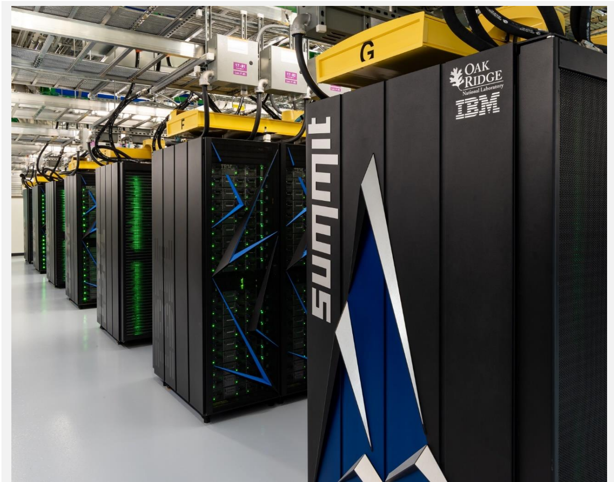
Figure X: ORNL Summit. Installed in 2018, Summit at the OLCF has held the No. 1 position on the TOP500 List four consecutive times. Using IBM Power9 CPUs and NVIDIA Tesla V100 GPUs, Summit achieved performance of 148.6 petaflop/s.
