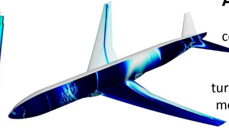
Simulation of a physical wind tunnel airplane model (the NASA Common Research Model), commonly used for CFD benchmarking and analysis.
