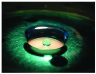
Superhydrophobic surface surrounded by a layer of water on an untreated surface *Photo courtesy of Oak Ridge National Laboratory*
