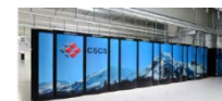
Piz Daint (Cray): Cray XC30 Intel Xeon E5-2670 8C 2.6 GHz Cray Aries NVIDIA K20x
