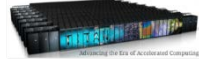
Titan (Cray): Cray XK7 AMD Opteron 6274 16C 2.2 GHz Cray Gemini NVIDIA K20x
