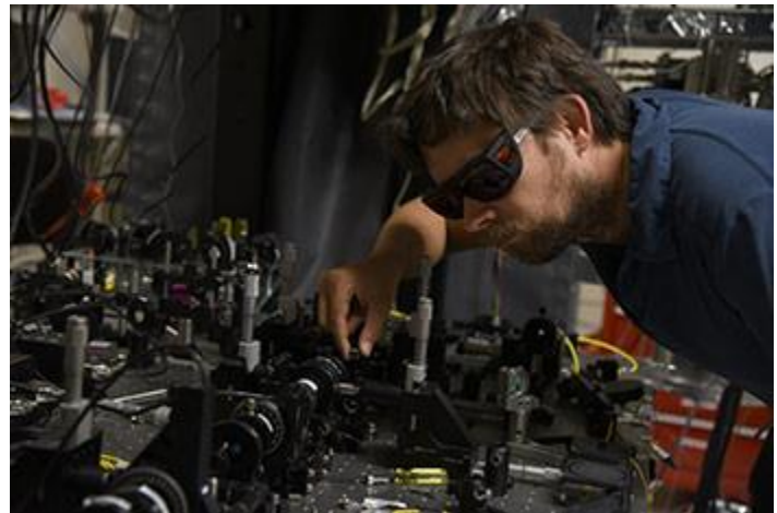
Figure 5. Physicist Krister Shalm with the photon source used in NIST's 2015 Bell test that strongly supports the existence of quantum entanglement. (Photo Credit: Burrus/NIST)
