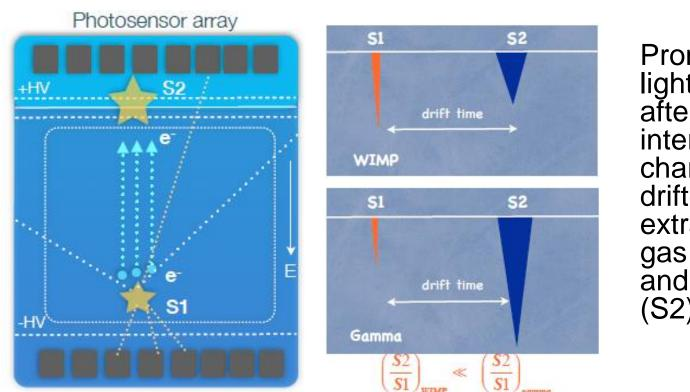
Prompt (S1) light signal after interaction; charge is drifted, extracted into gas phase and detected (S2)
