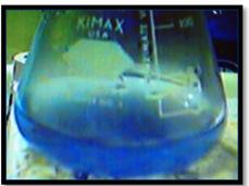
Proton-irradiated encapsulated Th target (left); Dissolved Th target showing blue Cerenkov glow (right).
