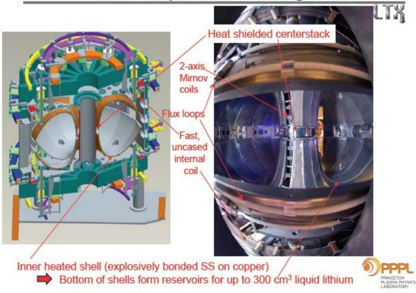
For magnetic fusion energy to fuel future power plants, scientists must find ways to control the interactions that take place between the volatile edge of the plasma and the walls that surround it in fusion facilities. Such interactions can profoundly affect conditions at the superhot core of the plasma in ways that include kicking up impurities that cool down the core and halt fusion reactions
