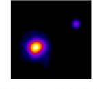
H8500 Hamamatsu 5cm x 5cm PSPMT – 2 mm thick BC408 plastic scintillator Cs137 & Cd109 electron sources
