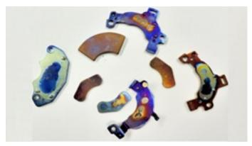
A photo of four voice coil magnets taken from a desktop or laptop computer and their brackets (which have mounting holes). These magnets are each about 10.5 - 15 grams, 1 - 1.25 inches long. These ones are colorful, because they have been overheated in the process of separation and demagnetization.
