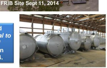
Five of fifteen nonconventional utility process tanks to be installed during conventional construction.
