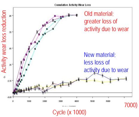
Cumulative 7Be activity wear loss versus wear cycles.
