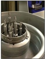
Mock-up core for the High Flux Isotope Reactor (HFIR) at Oak Ridge National Laboratory
