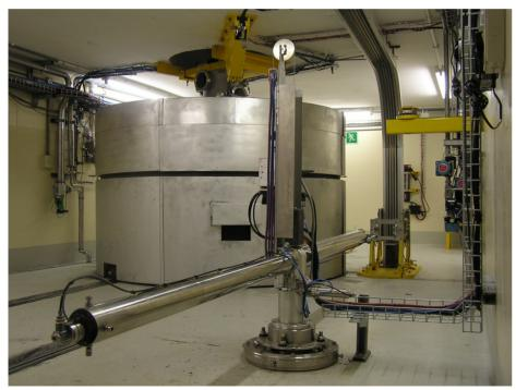
Vertical Beam Target Station (VBTS) 66 MeV proton beam with an intensity of ~250 µA
