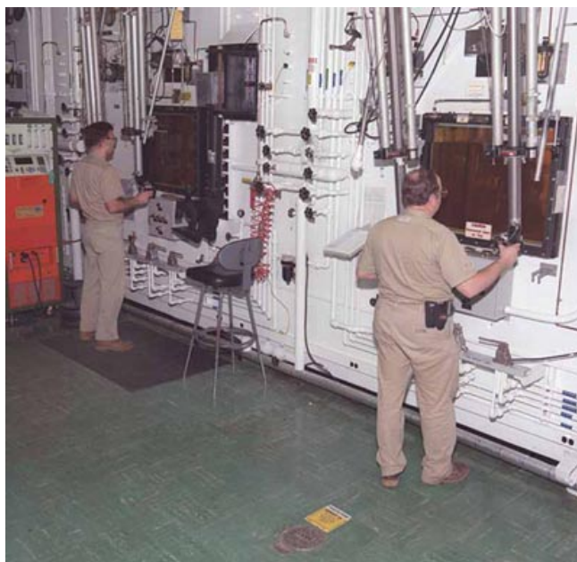
Several of Oak Ridge National Laboratory's hot cells are used in the processing and packaging a wide variety of medical and industrial isotopes.
