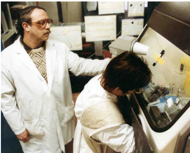
A health physicist monitors the dose rate at the window of a dedicated glove box at MURR, while a research technician formulates the Sm-153-labeled EDTMP which will be used to treat a dog with bone cancer.
