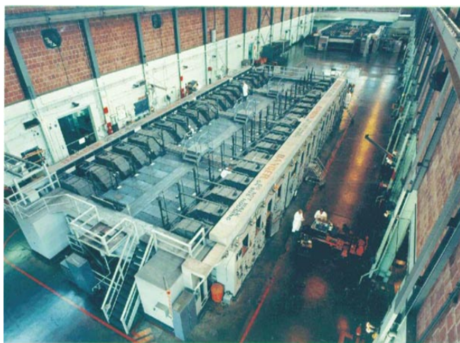
The large scale electromagnetic separators (Calutrons) at the Isotope Enrichment Facility (IEF) of Oak Ridge National Laboratory. They are the only large-scale separator of stable isotopes outside of Russia.
