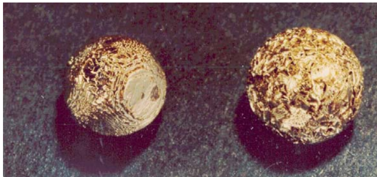
Magnesium Beads Grown Inside Still by Reduction/Distillation
